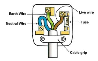
Ensure that the wires are secure and that no loose strands of conductor are exposed.
